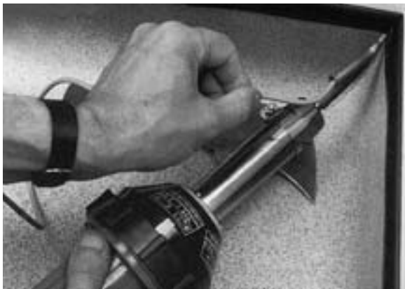
1. Groove the internal mitre before welding.
