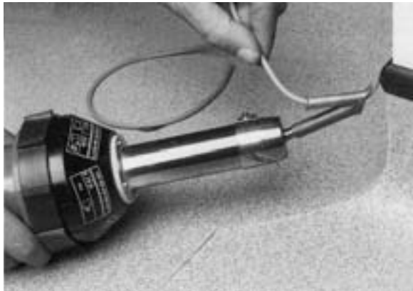
2. Start welding the mitre from the top, with the weldrod feed above the nozzle. When welding the floor feed the weldrod below the nozzle.
